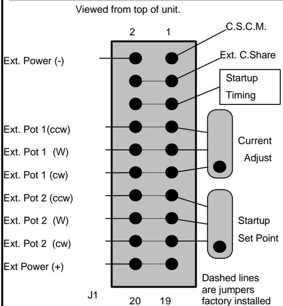
**Figure 3. Connector : Electrical Connections**
