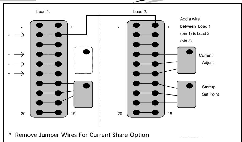
To add a **Power On-Off switch** remove the jumper on J1 pins 19 & 20 and replace that jumper with a switch. The switch must be capable of handling 250 mA. @ 12 VDC. **Note: DO NOT hook the power supply of one electronic load to the other!** To switch more than one load On-Off at a time, use a multi-pole switch.
